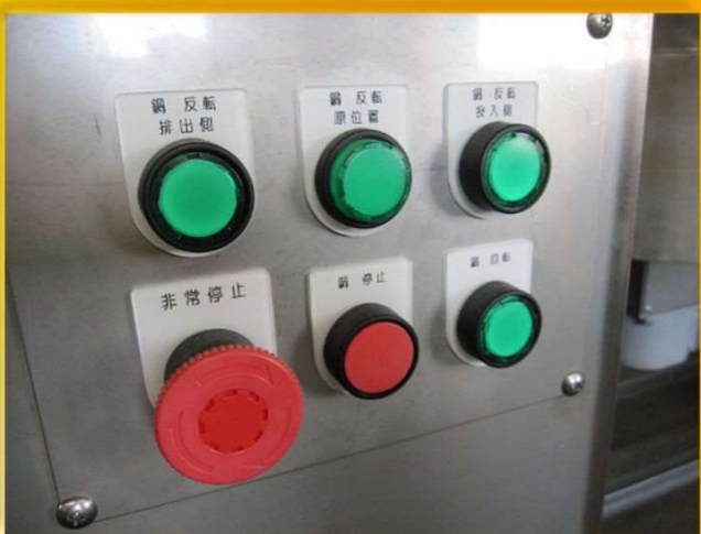
[Alternative Control Switches] Beside of Touch Panel, there are operation switches on unloading side.
