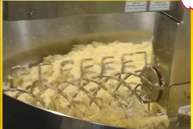
[Loosening & Mixing] By Special designed agitator and scraper, Food to be cooked as quick and uniform.
