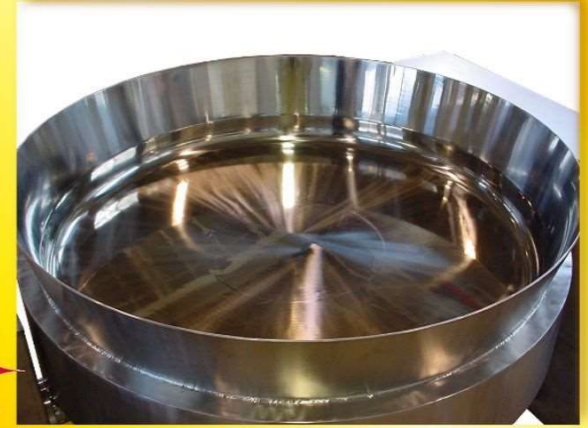
Stir-Frying by High Power Pan to be 1,100 mm dia. And 250 mm depth and optimum for Stir-Fry cooking.
